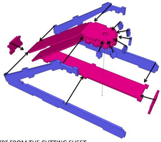
USE "A" OR "B" FROM THE CUTTING SHEET TO GET HORIZONTAL OR ANGLED ROTATION AXIS
